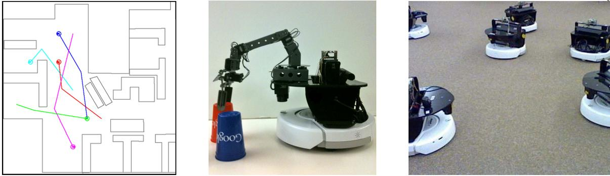
Figure 4.2: Left: 5 robots in an office environment and the resulting paths. Center and Right: Prairiedog platform. Each robot is equipped with an indoor localization system, a netbook and IEEE 802.11g wireless communication.
