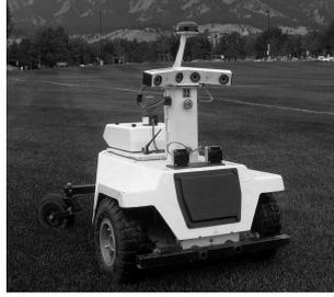
Figure 7: The LAGR robot platform.
